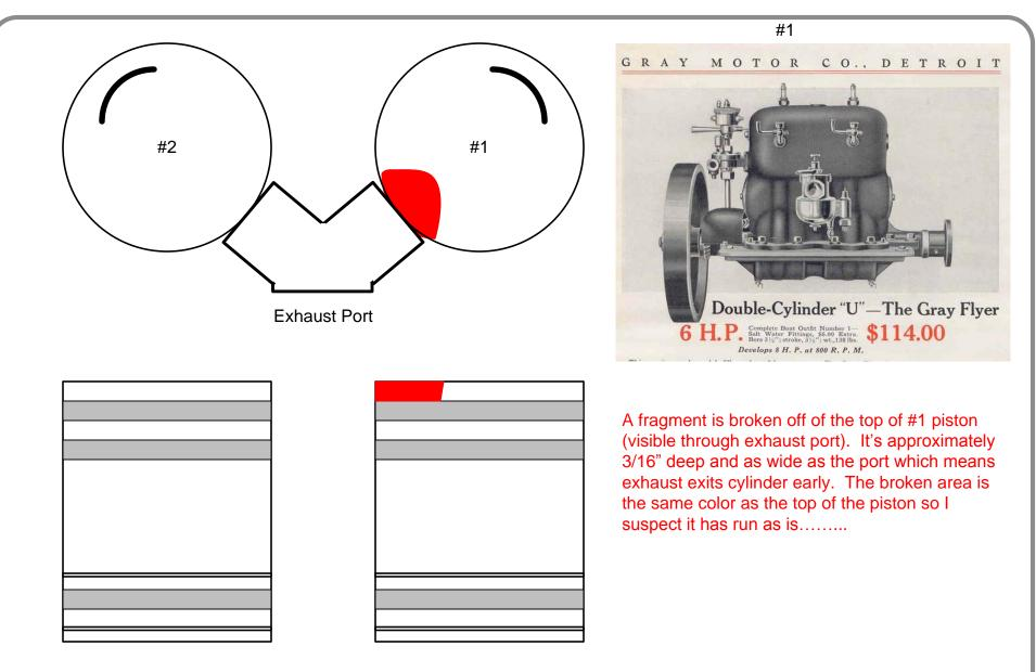
Engine is free. Using known good Schebler D carburetor and known good buzz coils. Trying to bump start against retarded spark. Engine will run occasionally but won't run for long. Very difficult to start. I really like this engine and would love to get it running well!
