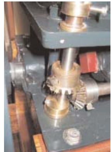
Right: Vertical timer shaft and new offset bearing.
