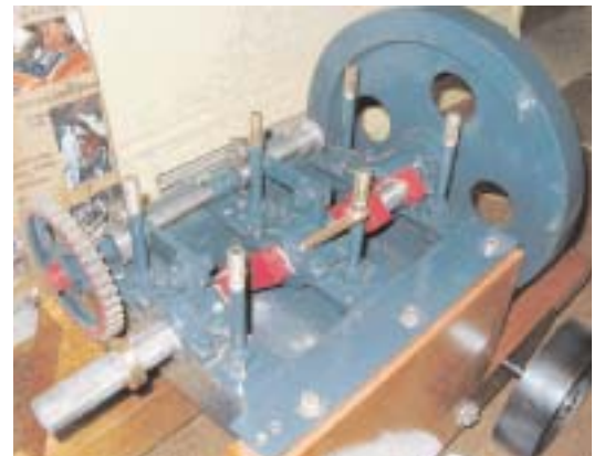
Right: The bedplate cleaned up with crank and camshaft fitted. Note the captive rollers riding on the cam. Neat stuff.
