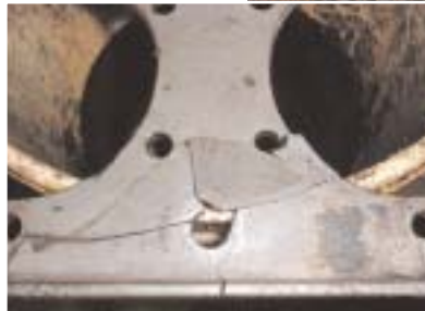
Above: Cracked and bent cylinder plate (note bent connecting rod). Left: Badly cracked cylinder plate. Below: Repaired cylinder plate.
