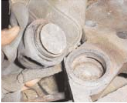
Above: Intake valve body removed from head, valve in place.
